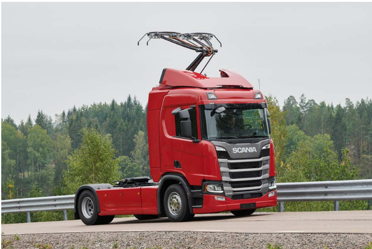
Figure 2: first Scania hybrid eHighway truck of the new generation
